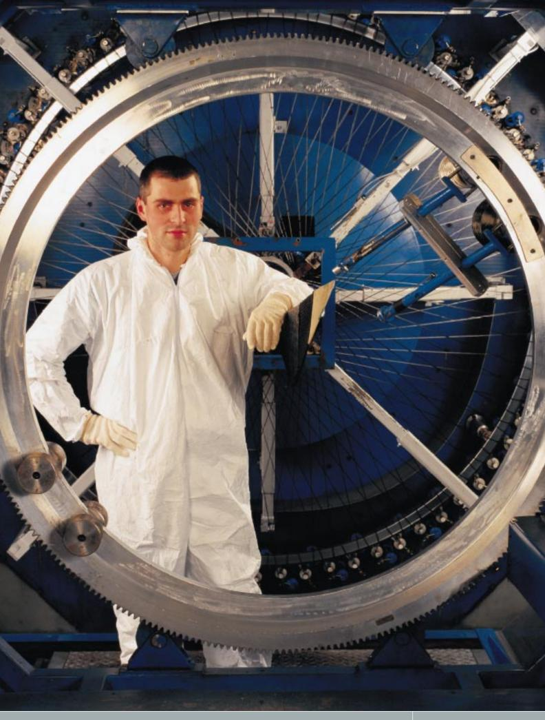
HAMILTON STANDARD—CATCH THE WIND "TO LEAVE A LIVING NAME BEHIND...AND WEAVE BUT NETS TO CATCH THE WIND." 17TH CENTURY BRITISH POET JOHN WEBSTER WOULD HAVE MADE A GREAT COPYWRITER FOR HAMILTON STANDARD'S RATIER-FIGEAC UNIT. BRAIDING-MACHINE OPERATORS THERE WRAP CARBON FIBERS TO FORM A PROPELLER THAT WILL TURN UP TO 1,200 RPMS, CATCH THE WIND AND LIFT A PLANE SKYWARD. POETRY IN MOTION.
