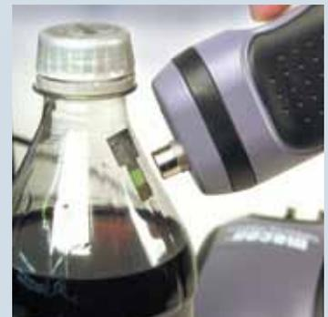
OpTech uses a fluorescence-based system for measuring total package integrity. The platinum sensor "fluoresces" or gives off light in an amount
