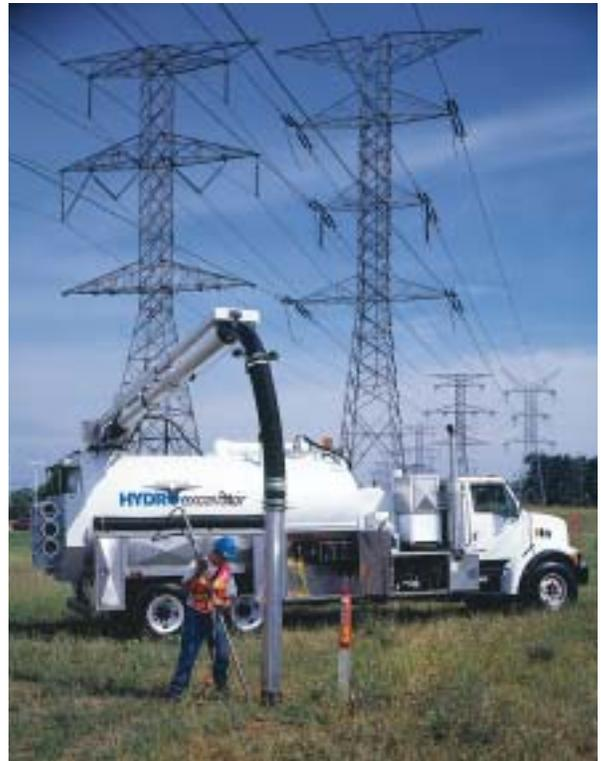
Uncovering buried utilities, natural gas and petroleum pipelines by traditional mechanical means can be complicated and dangerous. The Vactor HXX hydroexcavator makes excavating safer and more productive.
