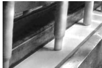
FC2 is dipped instead of welded for a seamless product.
